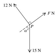
Three coplanar forces of magnitudes F N, 12 N and 15 N are in equilibrium acting at a point P in the directions shown in the diagram. Find  $\alpha$  and F. [4]
